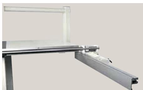
**The rip fence** has a cast iron body, extruded aluminium rule, and slides on a wide steel bar: there is no compromising on quality. The whole worktable can be easily and completely retracted.
