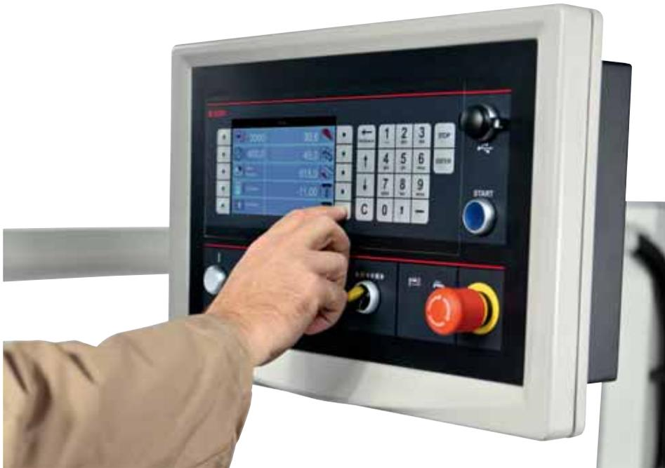
**The standard mobile upper control panel (only for SI400EP NOVA)**
