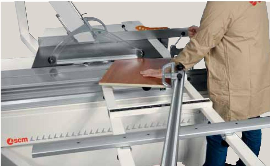
**Squaring fence** complete with two metal stops. The extruded aluminium structure grants the best precision. The smooth stops movement along the fence facilitates the set up.
